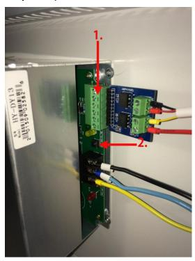
Press Test button, check if the Ammeter have reading and the laser tube will emit laser beam;
